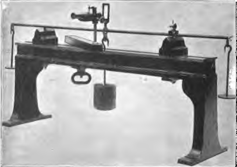
Fig. 39. Apparatus for measuring elasticity by deflection of beams.
